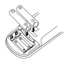
3. Place the cover over the compartment, press down lightly, and push it upward until it snaps on.
